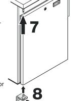
**8.** Insert hinge bracket in lower door mounting and screw into place.
