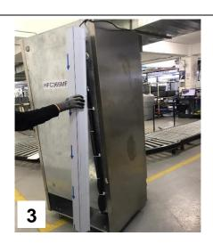
1-2-3) The back plate of the cabinet is disassembled by cordless or manual screwdriver and removed carefully.
