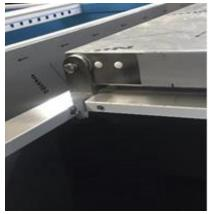
12. Push the top left door corner over the hinge bracket there and screw in the M8 screw.
