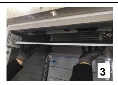
1-2-3) The inner air sheet plate of the refrigerator cabinet is disassembled by cordless or manual screwdriver and removed carefully.
