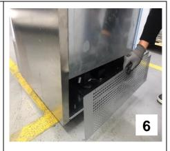
4-5-6) The lower back plate of the cabinet is disassembled by cordless or manual screwdriver and removed carefully.
