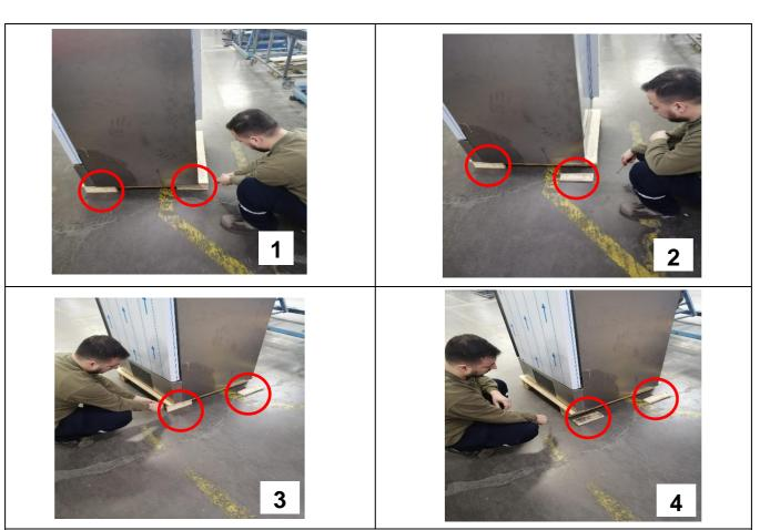
1-2-3-4) The blocking wooden pieces of the pallet (2 pieces) are removed by some sharp, flat edge tool (e.g. flat screwdriver) Once the pieces of wood that hold the cabinet to the pallet are removed, it means the cabinet is no longer connected to the pallet.
