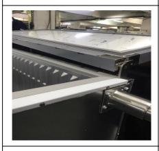
13. Screw in the fastening screws of the door closer at the bottom left.
