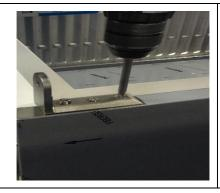
8. Move the hinges from the bottom right to the top left, and from the top right to the bottom left; PH2 screwdriver.
