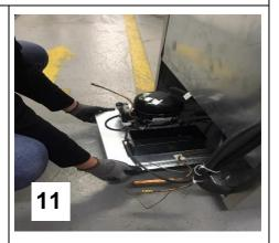
9-10-11) Condensing Unit is disassembled from where its mounted then dragged it out slowly.
