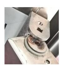
4. Remove the screw from the door closer square at the bottom right hinge. (wrench size 8 mm).
