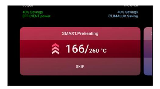
UNOX recommends that you use SMART. Preheating, an automatic preheating program that autonomously sets the preheating time and temperature; it also takes into account the dispersion of heat when you open the door and is activated when the oven moves from one step to the next, adjusting the oven cavity to the step's new parameters.
