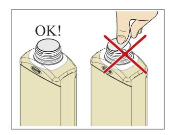
check that the protective film is intact and undamaged. Turn the bottle upside down and screw it onto the tank; a pin will break the protective film, which allows the detergent to pass safely into the tank.
