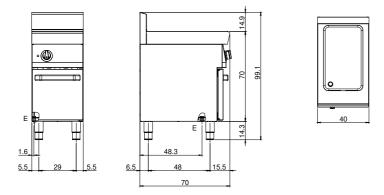
E: Electric power D: Drain for water H2O: Water inflow 3/4"
