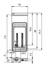
E: Electric power D: Drain for water H2O: Water inflow 3/4"
