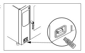
The USB interface is behind the cover on the bottom left of the housing.
