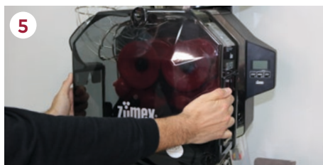
5 Turn the knobs 90° degrees until they are aligned with the holes in the cover. Then extract it.
