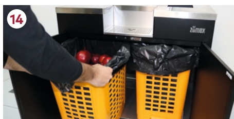
14 Remove the waste trolleys from the base to empty them.
