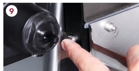
9 Press the side tabs to remove the bin .
