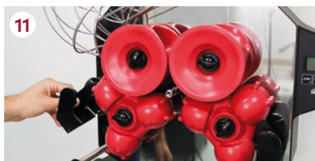
11 Pull off the peel ejectors.
