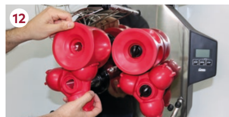
12 Unscrew the securing knobs of the pressing units. Take off the pressing units in pairs.
