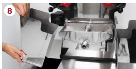
8 Remove the stainless-steel peel guides .
