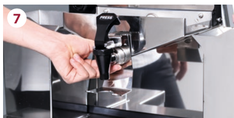
7 Remove the Speed Up Tap by easily unscrewing it.
