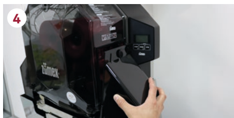
4 Turn the knobs towards us counterclockwise to their vertical position and extract the side outlets.
