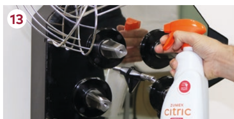
13 Clean the front zone of the machine, following the steps shown and removing all the particles which have adhered.
